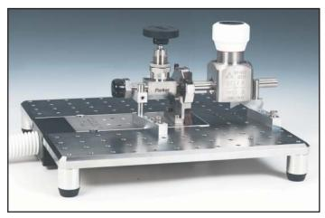
The available fixturing/positioning plate is provided with an assortment of supports and fixture blocks. This tooling facilitates rapid and repeatable alignment and positioning of multiple welded components.
