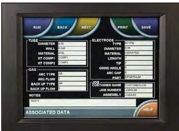
For jobs that require supporting data, the Model 205 provides fields for recording a variety of associated data. Details pertaining to the gas, the electrode, the components being welded and specifics about the job or customer can be stored with each weld schedule.
