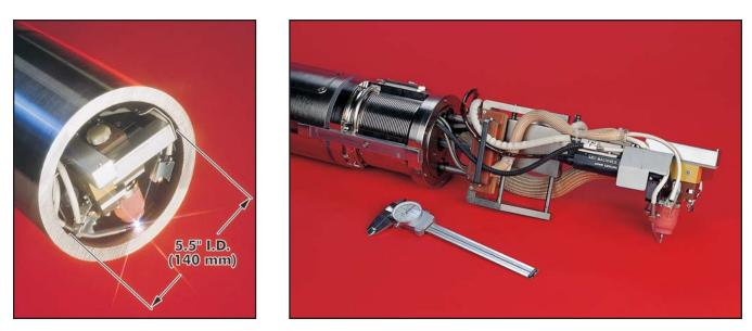
The Model 73 weld head is designed to make butt weld, cladding and weld overlay repairs by remote control on the inside diameters (I.D.) of piping and specialized valve systems. The Model 73 is a smaller version of the industry standard Model 43 weld head for applications in reduced diameters.
