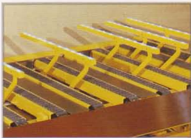
Bar-type sheet supports
