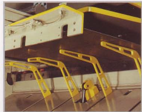
Pneumatic sheet supports
