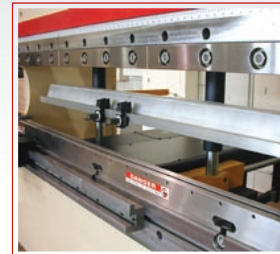
CNC backgate for 90 - 175 ton, 6' and 8' machines
