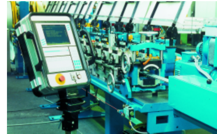
Rollforming machine for light profiles
