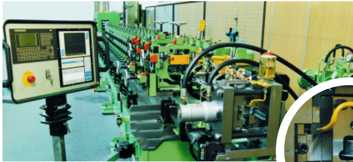
High precision in Start-Stop® operation for manufacturing electrical enclosure profiles
