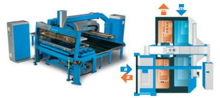
Compact Express is a fully automated material handling device. The placing of the automatic loading and unloading unit makes it possible to use several combinations of automatic and manual loading and unloading cycles. The manual loading table is free for use for manual operation.
