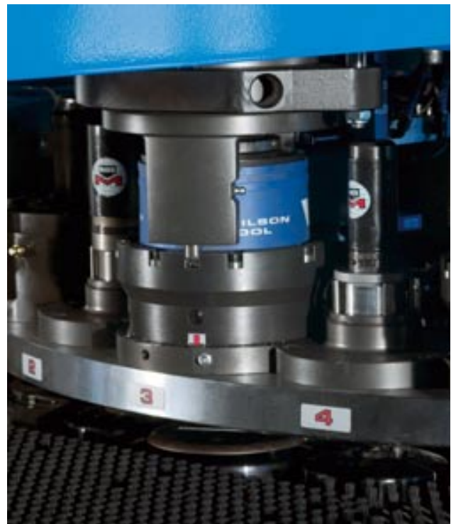
Example of a customer specific turret layout. This one includes 66 tools, of which seven index tools and one indexable high-forming station.
