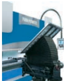
Right, top: E-Bend L uses a laser beam in measuring. Right, bottom: E-Bend M has sensors to assure constant quality.
