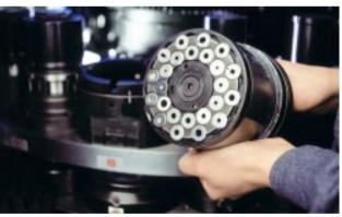
The turret can be equipped with **MultiTool\*** stations to increase the number of tools. The MultiTool\* station is mounted on the turret like a normal tool station and the tools are mounted in rapidly changeable punch and die cassettes, which are available also as additional equipment.
