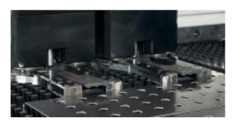
The clamps are equipped with sheet detecting sensors, which continuously monitor sheet security in the clamp, ensuring accuracy and reliable machine operation.
