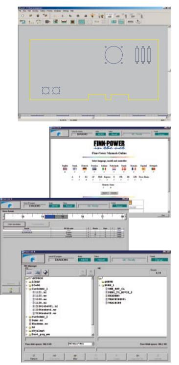
NC Express with its easy-to-use 2D-CAD, advanced auto tool placement, automatic nesting and optimizer, parametric programs as well as a versatile interface for order management aims to minimize programming times, which means higher machine utilization especially in short-run production.
