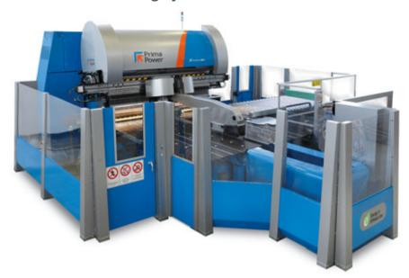
Prima Power's BCe series bending centres offer the well-known express bender benefits – precision, flexibility and high surface quality in a semi-automatic process. Only loading is performed manually – an easy task due to user-friendly design.
