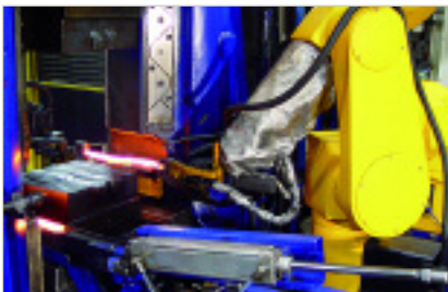
Longer blanks can be forged in multiple impressions using LASCO grippers.
