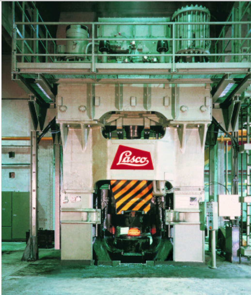
LASCO GH 2500, 250 kJ blow energy, weight: approx. 150 000 kg, programmable control.
