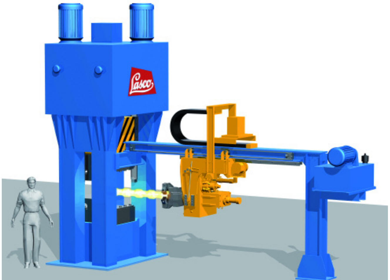
LASCO AR 250 stretching unit consisting of a VPE 250 hydraulic press and a stretching manipulator.
