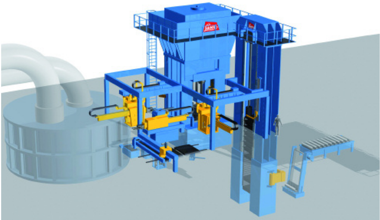
Fully automatic production line with VPA 2500 and VPA 315 hydraulic presses from LASCO.
