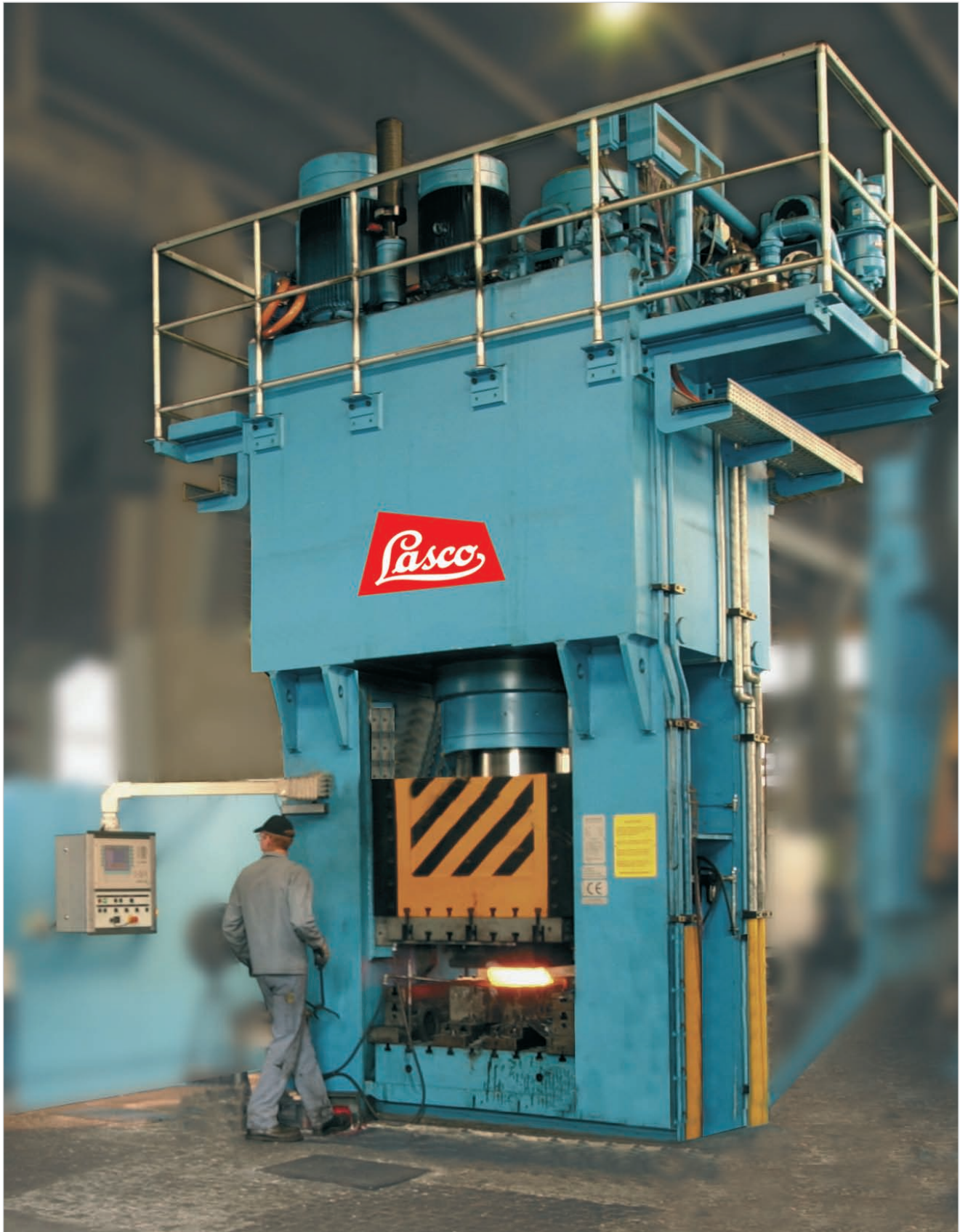
A billet is pre-formed for a ring, on a VPE 800.
