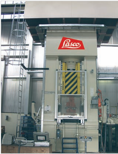
KFP 1000 forming aluminium parts for the automotive industry.
