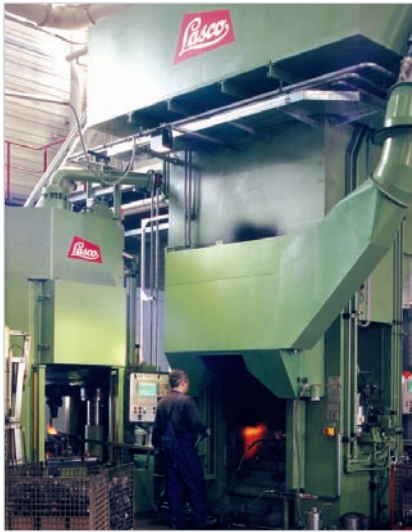
Pistons are forged on a VPE 160 and a VP 800.
