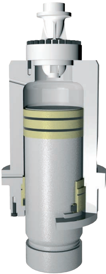
Layout of a press cylinder on a "LASCO" hydraulic press.
