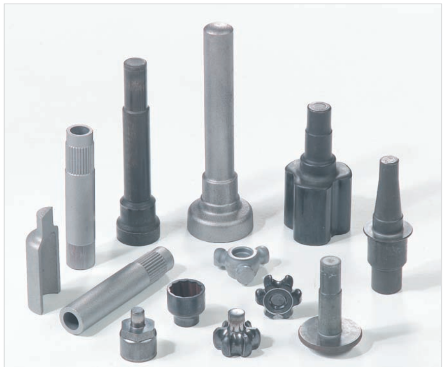
Typical parts produced by LASCO hydraulic KFP cold extrusion presses.
