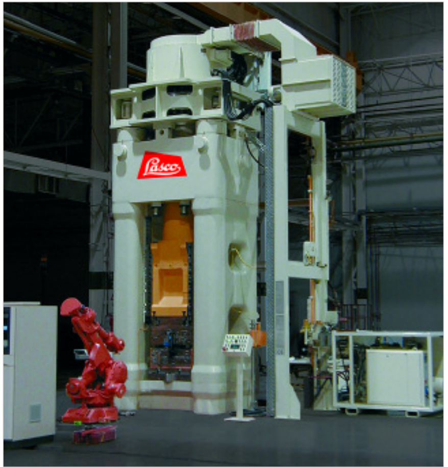
The automated LASCO SPR 1250 screw press working in the facility of an automotive supplier in the USA.
