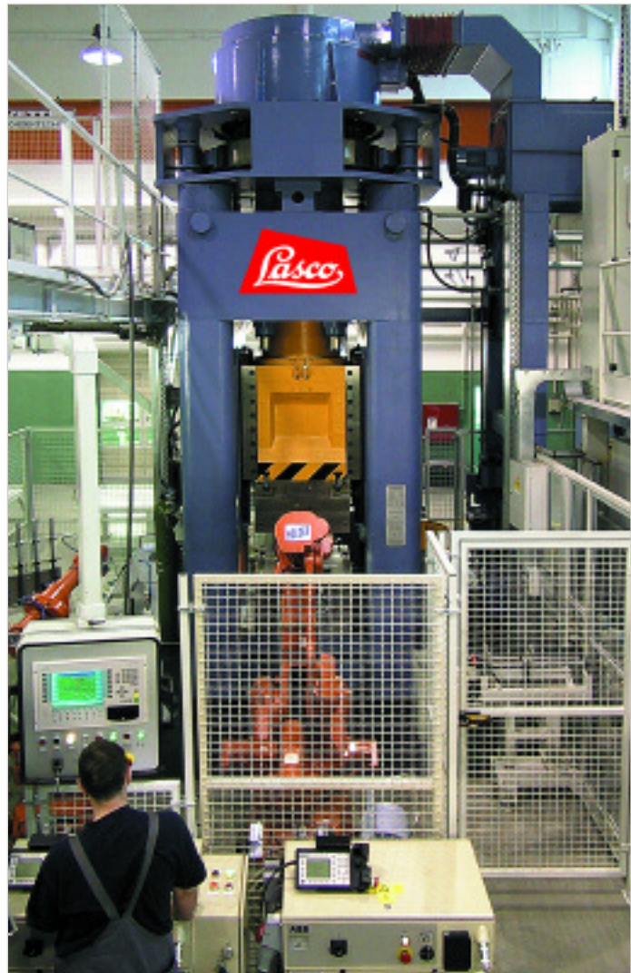
LASCO screw presses with frequency converter drive are in use worldwide. In the illustration, racks for automotive steering racks are being produced on an automated SPR 1000.
