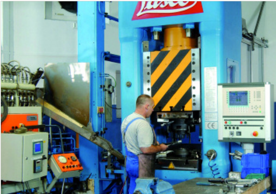
An SPR 400 screw press used for production of electric armatures for railroad vehicles. The preheated blanks in the furnace (left) are fed to the machine through a chute.
