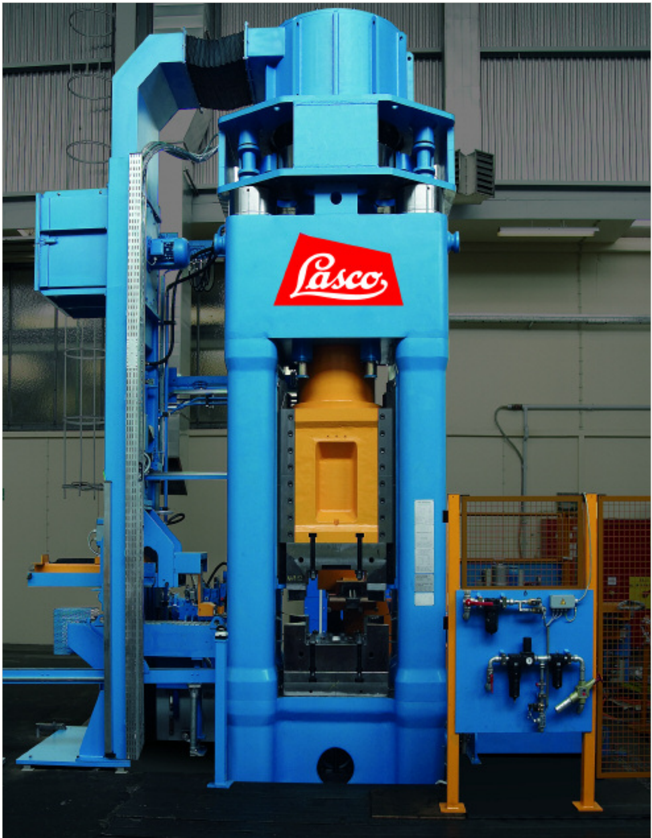
Fully automated production of vehicle components on a LASCO SPR 1000.
