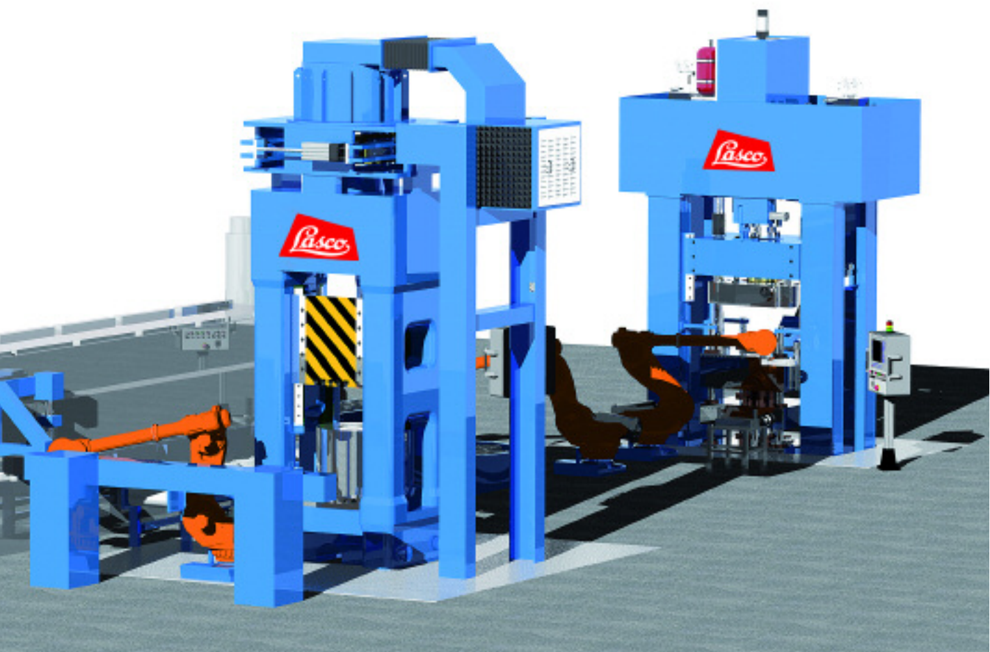
Schematic of two interlinked LASCO units SPR 630 and MPP 400 with automation devices.
