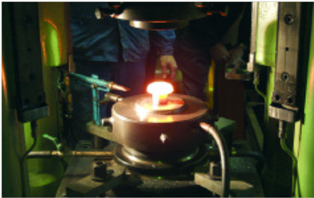
Production of connecting elements on an SPR 315.
