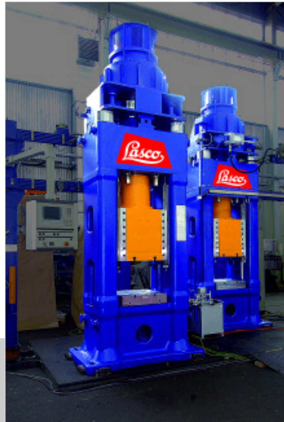
Two LASCO SPP 400 in the assembly hall.
