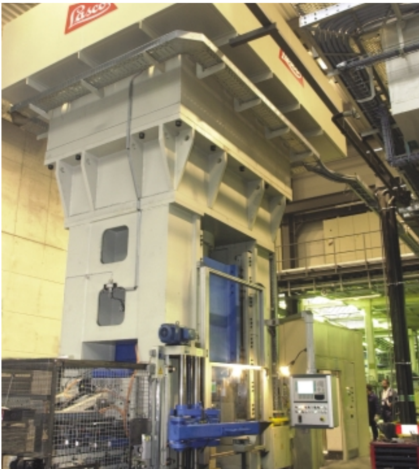
Cold extrusion press KFP 1000.
