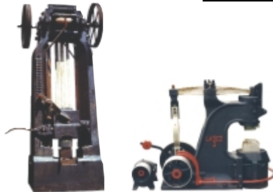
Historical LASCO innovations: board drop hammer (left) and spring hammer (right), both built before 1900.
