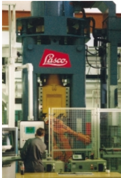
Fully automatic production of steering gears in a screw press SPR 1000.
