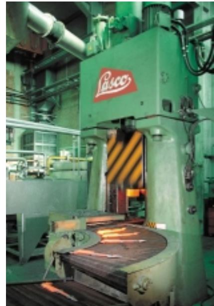
The die forging hammer type HO-U 200 forges hand tools
