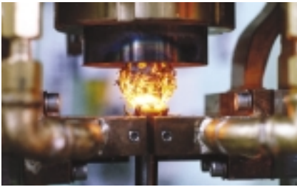
Electric upsetting (valve).
