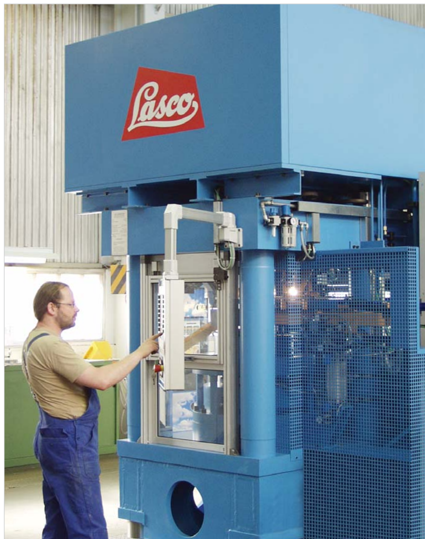
LASCO UK 500 upstroking compact press for the manufacture of carrier plates.
