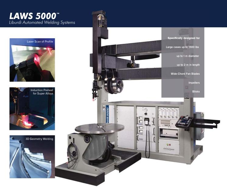
The LAWS-5000™ 5-7 axis, fully coordinated motion welding system offers computer synchronized pulsing of the wire and current to yield exceptional heat management at the torch. This unequalled heat management feature allows the LAWS-5000™ to process critical aerospace parts like thin knife edge seals, turbine cases and combustor liners with superior results.
