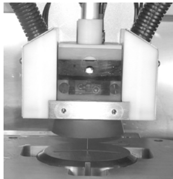
Photo 2: Advanced wire EDM machine producing a shaped thick turret die.
