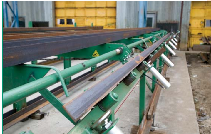
Loading stock from either direction – outside the building – and then passing through a small opening in your wall saves valuable shop floor space.
