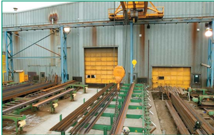
Loading stock from either direction – outside the building – and then passing through a small opening in your wall saves valuable shop floor space.
