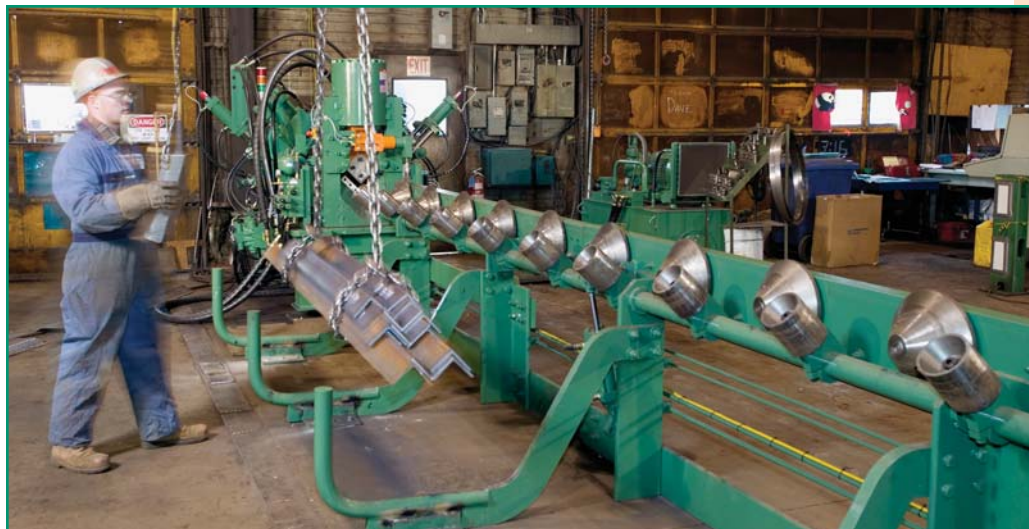
Punch, shear, position and unload angle and flat stock in one operation.
