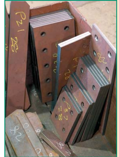
With 12 x 1" (305 x 25mm) capacity, base plates are processed in a simple one pass process.
