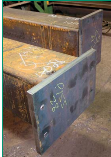
With 12 x 1" (305 x 25mm) capacity, base plates are processed in a simple one pass process.
