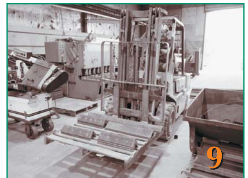
Move pieces to punch area.
