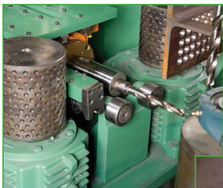
The integrated Signoscript carbide marking system provides legible part identification.
