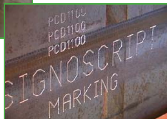
The integrated Signoscript carbide marking system provides legible part identification.
