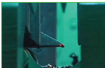
Laser referencing, even for the most pronounced miter sections, insures pinpoint accuracy.
