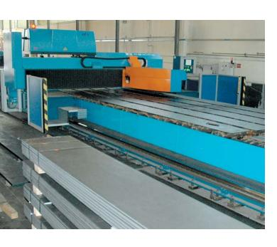
The piece remains fixed during the work process: it is the machine that moves to reach the area to be machined.
