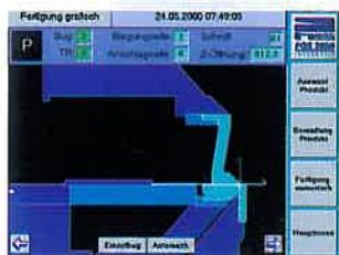
The bending machine, workpiece and tools are represented schematically and updated for every bending step. All actions to be performed by the operator, such as turning, rotating, etc. are displayed for each bending step, to provide optimum support for even the most inexperienced of machine operators.
