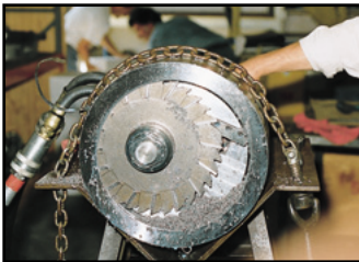
Solution Profile: When it comes to completely custom pipe cutting machinery, customers depend on Tri Tool's special engineering as was the case with this ID mounted saw which cut from the bore out.
