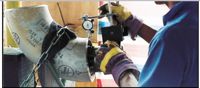
Solution Profile: An elbow mandrel head being mounted in a fitting and being aligned with a dial indicator for maximum precision.
