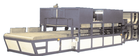
ROLL-JET™ RJ 710 Automatic Rolling Table for cutting of Fibreglass Rolls 2.000 mm x 3.000 mm (7' x 10').
