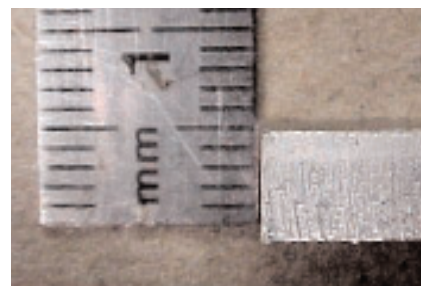
6 mm thick ALUMINUM cut with PURE WATER ONLY
