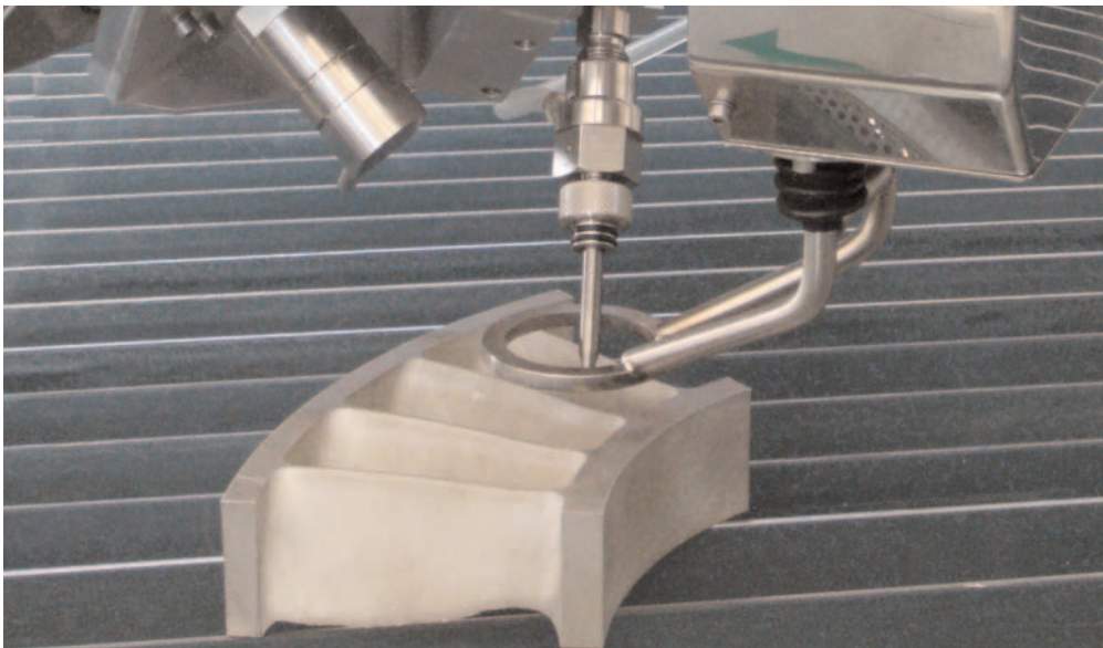
5 axis 2D inclined cutting with touch probe
